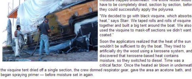
moisture trapped underneath. The entire vessel would have to be completely dried, section by section, before they could successfully apply the polyurea. We decided to go with black visquine, which absorbs heat," says Starr. We taped rolls and rolls of visquine
